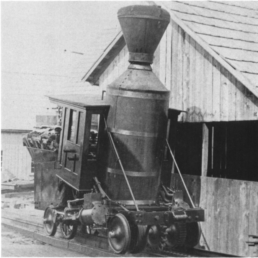
Figure 7. Cog Railway locomotive first #3 resting on the original strap-iron rails at the Base Station, c1870. Courtesy of the New Hampshire Historical Society, stereograph S23.
