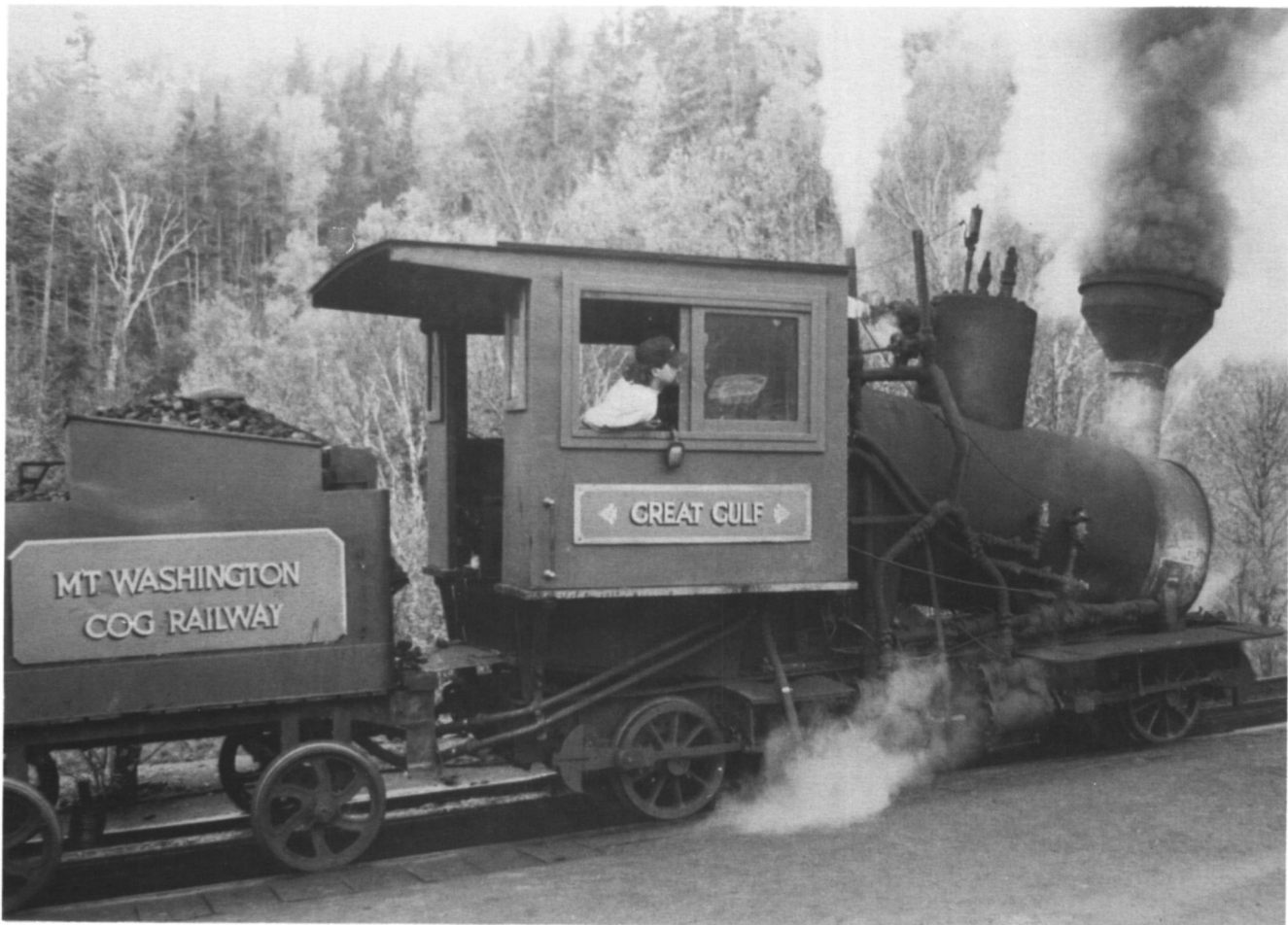
Figure 22. Cog Railway locomotive, the current #6 (Great Gulf), at the Base Station, 1994. Great clouds of steam are generated by the boiler, which is under a lot of pressure. Photo by the author.
