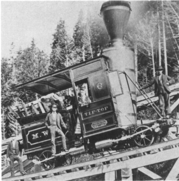
Figure 13. Cog Railway locomotive first #6 (Tip Top) just after leaving the Base Station, c1874. This was the first locomotive with four cylinders and a cab roof overhang. The builder's plate on the side of the cab reads: "Manchester Locomotive Works, N.H.-1874." Trestle work from the original track may be seen behind the locomotive. Courtesy of the New Hampshire Historical Society, stereograph S27.
