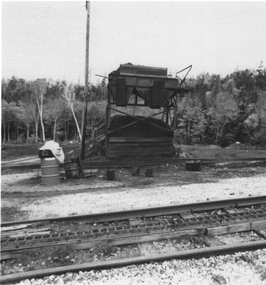
Figure 26. The coal loader at the Base Station that fills the coal tenders, 1994. Photo by the author.
