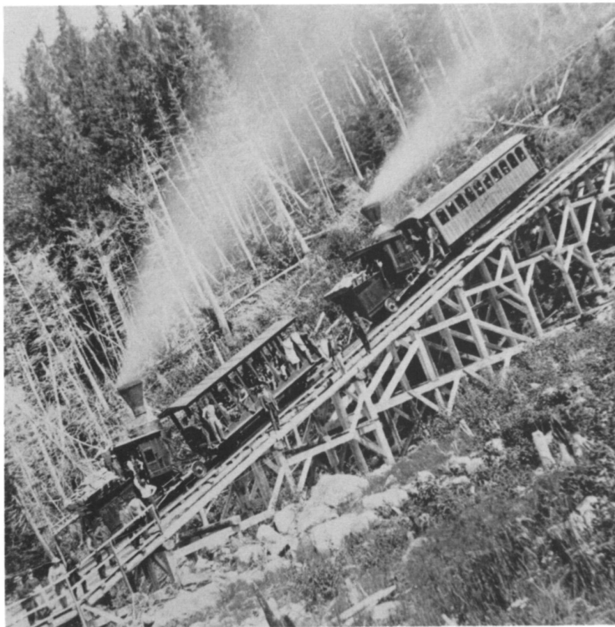
Figure 11. Cog Railway locomotive second #2 (George Stephenson) with first "open" coach (at left), and locomotive first #3 with "closed" coach (at right), just after leaving the Base Station, c1869-70. Courtesy of the New Hampshire Historical Society, stereograph S13.
