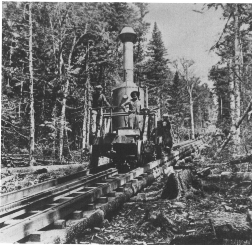
Figure 5. Old Peppersass with a flatcar load of passengers, c1867. Photo taken before the addition of a fuel and water bunker on the rear of the locomotive. The individuals standing by the boiler are probably Daniel Kidder and Charles Aiken (right), early mechanics and engineers of the railway. Courtesy of the New Hampshire Historical Society, stereograph S21.
