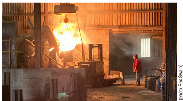
Fig 6. Molten iron pouring from the furnace into a bucket, or crucible, to be transported to the flasks
