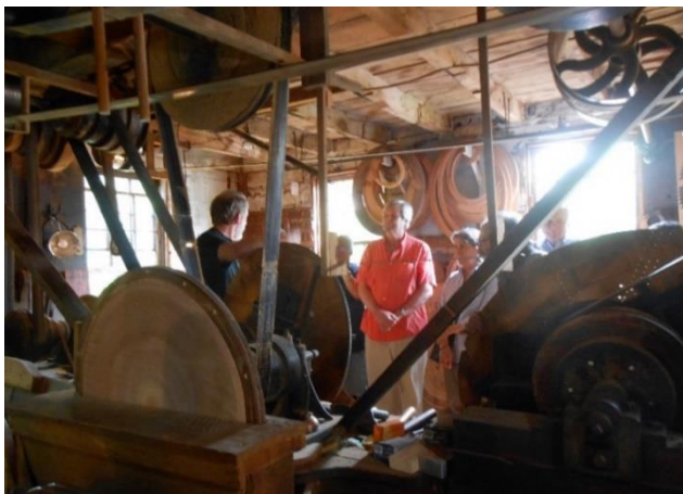
The oval turning lathes, driven by flat belts. (Betsey Dexter Dyer)
