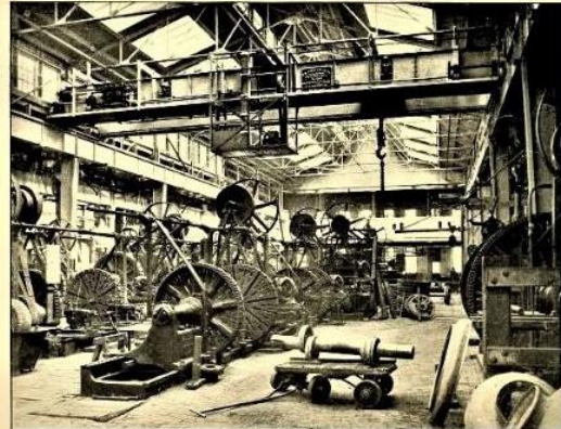
10-TON TRAVELLING CRANE. IN WHEEL-SHOP, BALDWIN LOCOMOTIVE WORKS.
