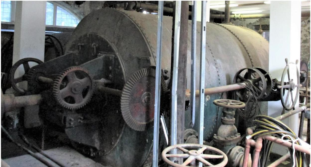
*View of turbine from the other side. We believe the water leaves in the bottom of the turbine and that the gears control the wicket gates.*
