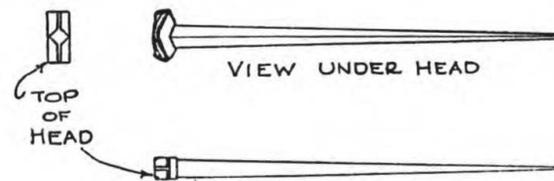
*Diagram of a 1799 Perkins-manufactured nail.
