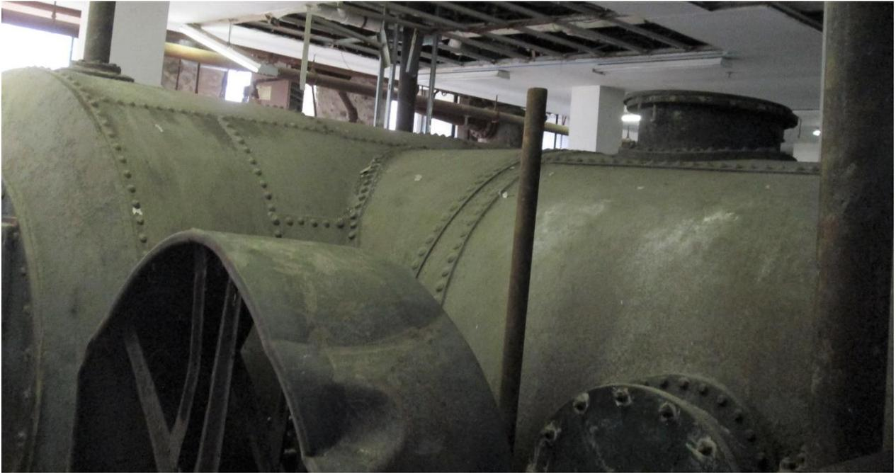
*Overall view of the turbine. Water enters from the right and splits to drive what appear to be two turbines at the left. We think the water exits below the turbine. In the foreground is a battered flat belt pulley.*
