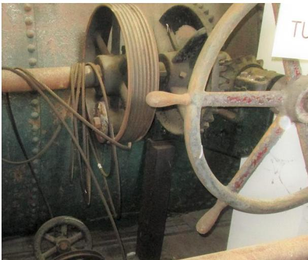
*Left: Closeup of the control shaft, showing the drum that connects the turbine control shaft to the governor via cables and the cable sheaves on the floor.*
