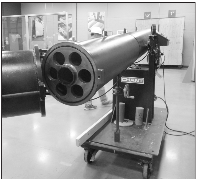
A view of the breach of the compressed air cannon that is used to fire 2x4s into sheets of plywood, demonstrating the effects of wind-borne debris on wall materials. The 2x4 went right through the 1/2 inch plywood, while the 1-inch thick plywood safely repelled the lumber missile.
