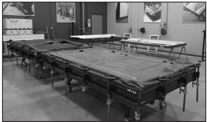
Testing tables within the Natural Hazards Laboratory for demonstrating the effects of wind uplift on membrane roofing.
