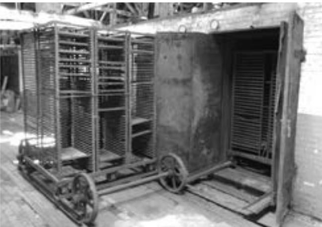
*A view of the oven and trolley system inside the paint shop (aka "Japanning house"). Freshly painted items were placed on metal trays and onto the racks. A two-way track system allowed the carts to be rolled directly into the drying ovens. The tracks extend into a nearby storage room. This building contains twelve of these large ovens, and several smaller ovens in which the trays are loaded in by hand. It also contains belt-driven mixing drums where the paint was applied to the products.*
