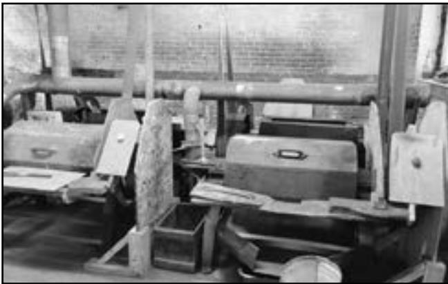
*View of the "rattler room". Freshly painted metal items are loaded into the belt-driven drums with sawdust and rolled to remove bumps and provide a smooth finish to the products.*
