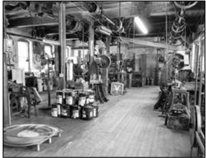
*A view of the “main shop” containing an array of antique machinery (mostly small presses), modified slightly over the years to produce a variety of small metal items such as insulated staples and cable clamps for telephone and electrical wiring. The machines in this room are still run by an overhead shaft-and-belt system – originally powered by a steam engine in an adjacent building, it is now operated by antique electric motors.*
