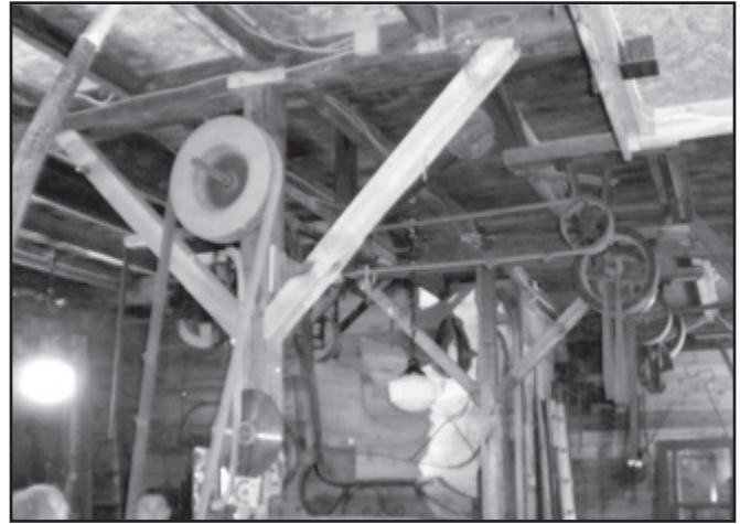
The belt and pulley system for the Sleigh Mill's sanding drum.
