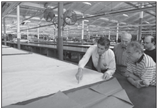
Joseph Abboud Manufacturing Company President Anthony Sapienza explains the layout and cutting process. There are about one hundred separate pieces that go into a men's suit, each is given a number to ensure it is routed to the correct sewing station for assembly, in the correct order – a challenging task with almost 1,200 suits per day of various sizes, colors and designs.
