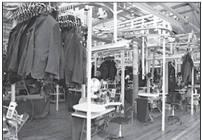
The automated Eton System at Joseph Abboud Manufacturing Company. Used to deliver suit coats in various stages of production to the correct terminal for assembly. Each sewing station in the factory is tied into a real-time shop-floor control software system that tracks the production of each worker.
