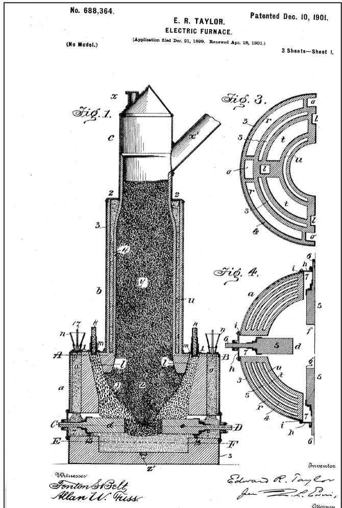
Figure 2. A Drawing of an electric furnace published in Edward R. Taylor's patent filed in 1899.
