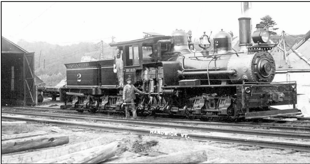
Figure 4. Shay Geared Locomotive No. 2, Hardwick & Woodbury RR, Hardwick, VT.
