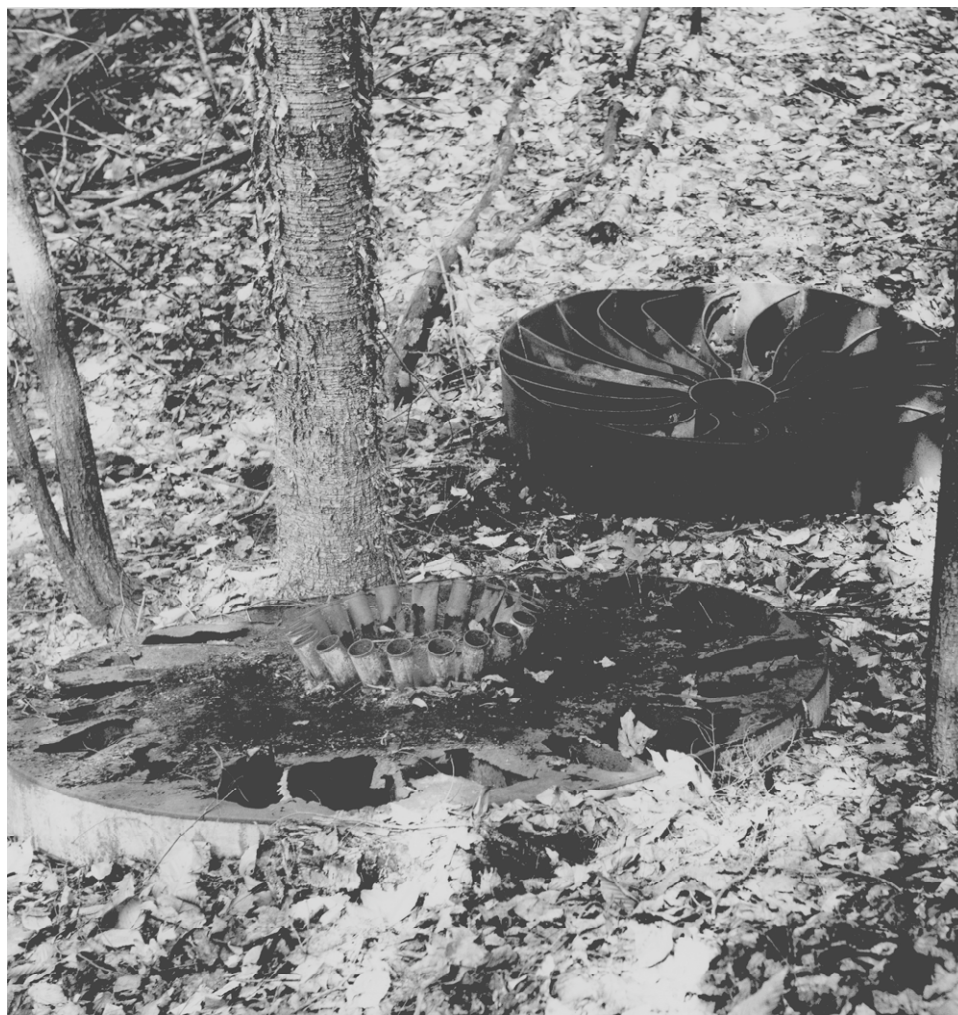
Buddle components at concentrating mill. Photographed by Suzette Usher.
