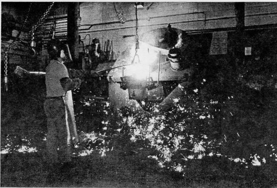
Sparks fly as a Belcher foundryman fills a ladle with molten iron from a tilting induction melting furnace.
